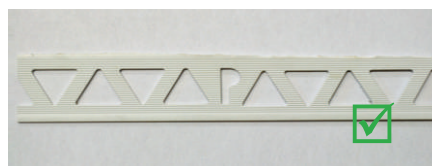
PTT RENDER Trims & Angles perform superbly after exposure to 1000 hours of UV testing, according to ASTM G154
