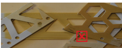
Bad discolouration at just 200 hours of the UV test ASTM G154
